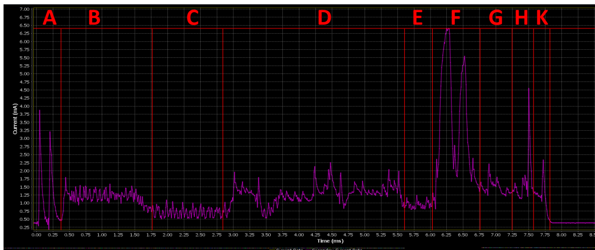
Figure 125: BLE Connection power profile
