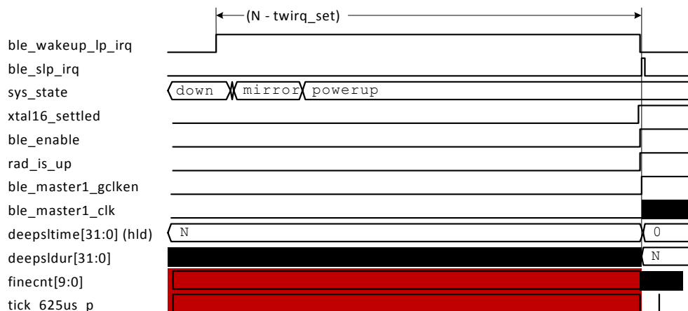
Figure 121: Exit BLE Deep Sleep Mode at predetermined time (zoom out)
