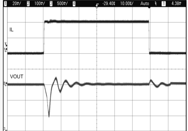
Figure 25. Load Transient, 0 mA to 400 mA, V_{OUT} = 2.5\text{ V} in Low-Power Mode
