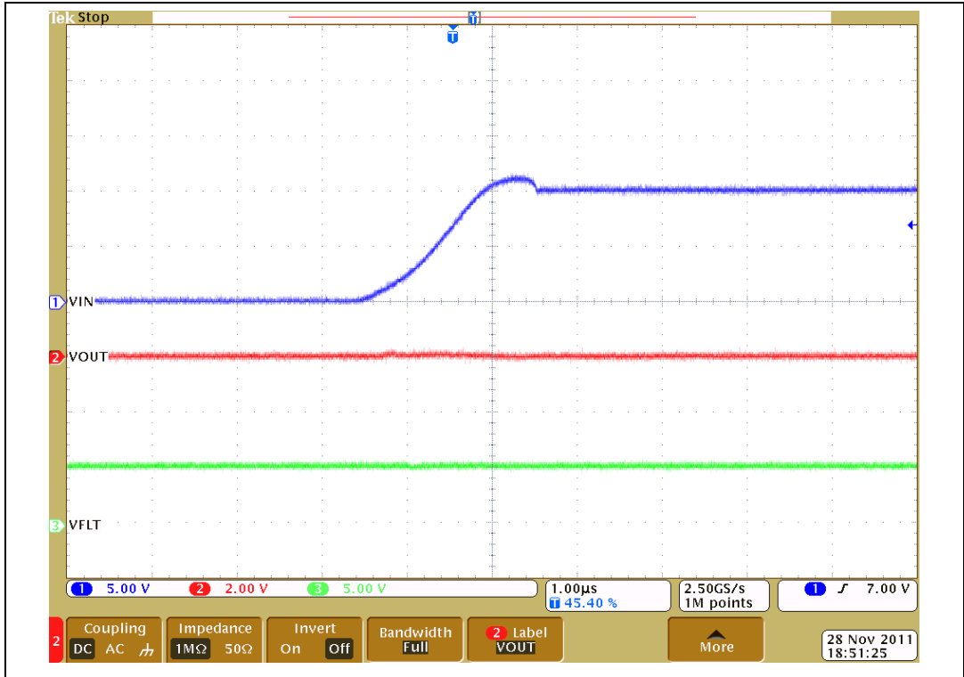
Figure 15. Startup to overvoltage (detail)
